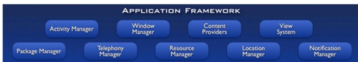
Figure 5: Application Framework Layer
