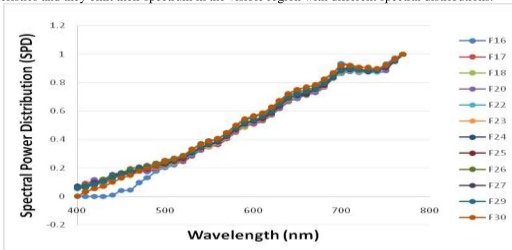
**Figure 3.** the spectral power distribution of some working standard lamps.
