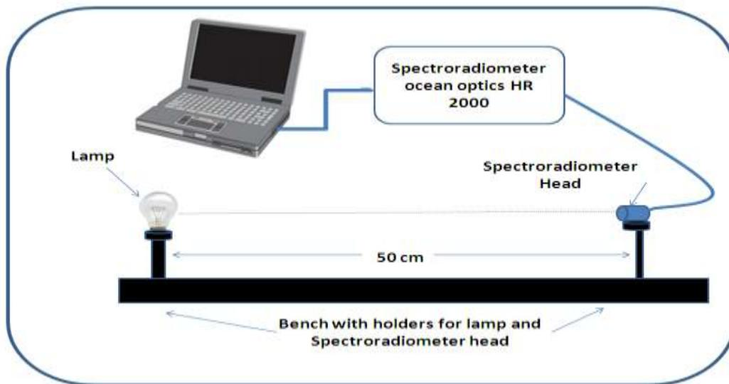
**Figure 2.** Set up of measuring the spectral power distribution of NIS total luminous flux secondary and working standard lamps.
