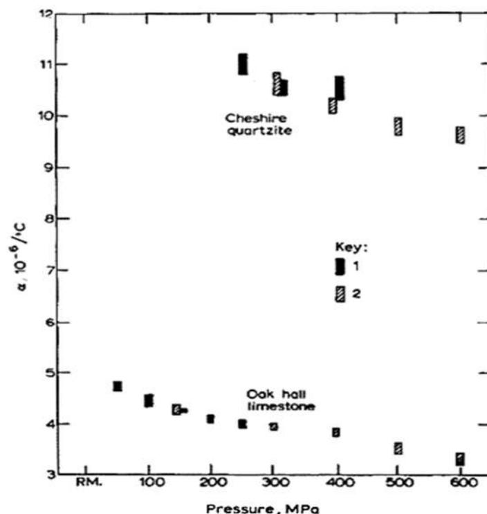
**Figure 2:** Influence of confining pressure on thermal expansion- when pressure was (1) decreased and (2) increased (Wong and Brace, 1979).
