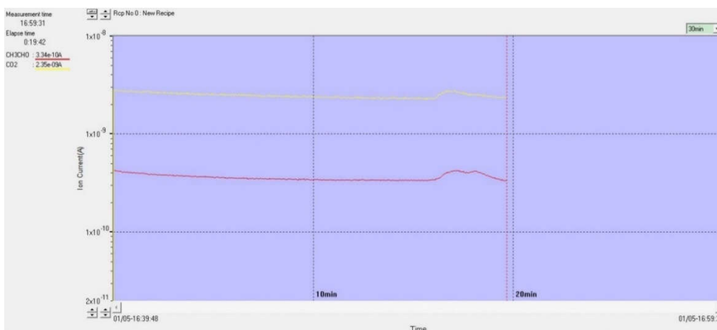
Fig. 7. Reality spectra of m/z=29 and m/z=44 for the ethanol oxidation on Pt/C.
