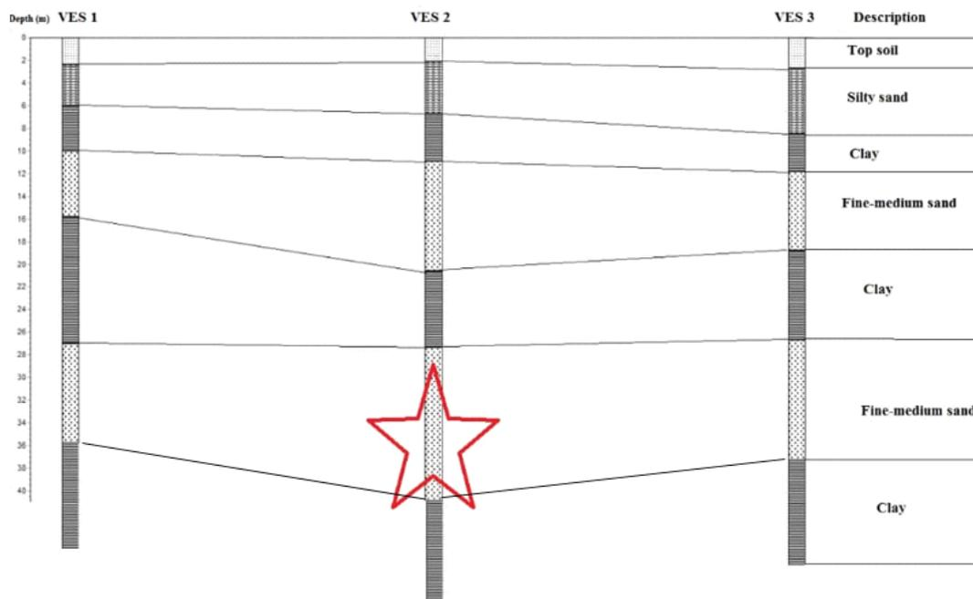
Fig. 5 2D geo-electric cross-section over sampled area showing recommended drilling target
