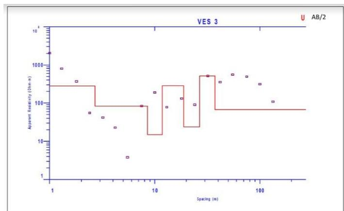
Fig. 4 VES 3 geo-electric curve
