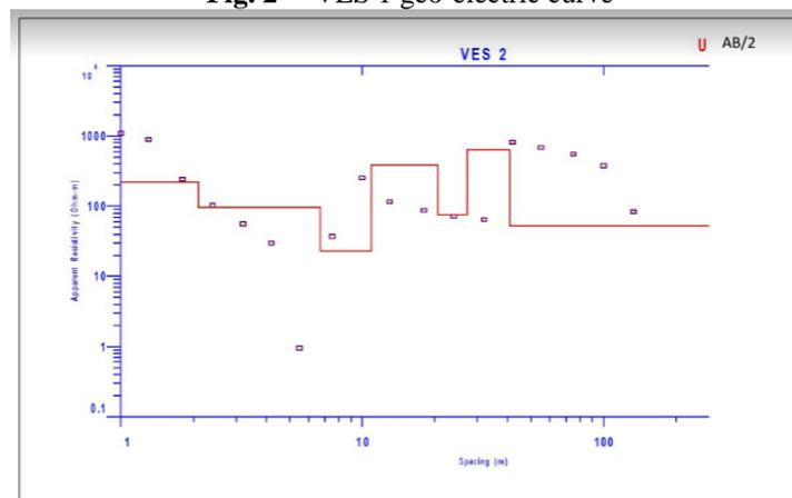
Fig. 3 VES 2 geo-electric curve
