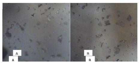
Fig.3.Morphology of PVA(S) (A) and PVA-ECH (B) seen by polarizing optical microscopy at (x100)
