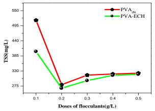
Fig.5. Evolution of the TSS of effluents treated with  $\ensuremath{\text{PVA}}_{(S)}$  and  $\ensuremath{\text{PVA}}\xspace$ -ECH
