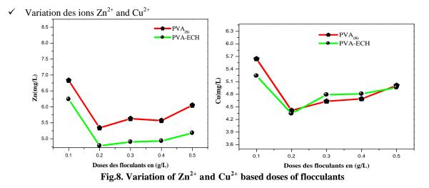
From the curves shown in Figure 8 we found that the gradual increase in flocculant doses applied, slightly decreases the zinc and copper contents of the treated effluents, such as the  $Zn^{2+}$  and  $Cu^{2+}$  values, were respectively recorded in 5.34; 4.78; and 4.414; 4.34mg/L at a dose of 0.2g/L PVA<sub>(S)</sub>, PVA-ECH successively.
