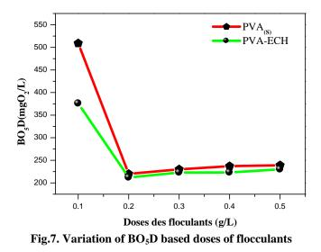
From this figure, we found that  $BO_5D$  has decreased from 602mg/L to minimum values of the order of 220; 212mgO<sub>2</sub>/L for optimal dose of 0.2g/L the PVA<sub>(8)</sub> and PVA-ECH successively.
