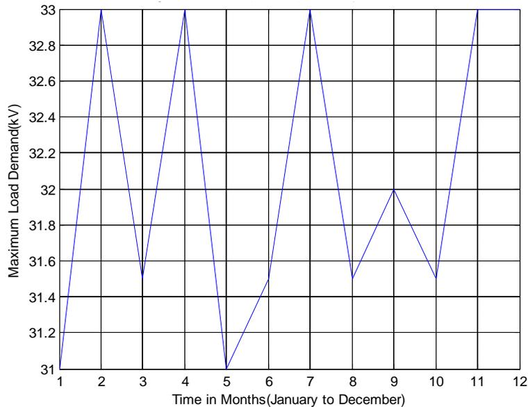
Fig.7: peak voltage versus time (in months) on Owerri feeder from Jan. to Dec., 2012.
