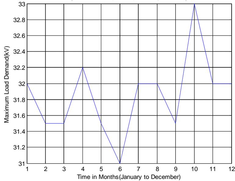
Fig.8: peak voltage versus time (in months) on Ogotu feeder from Jan. to Dec., 2012.
