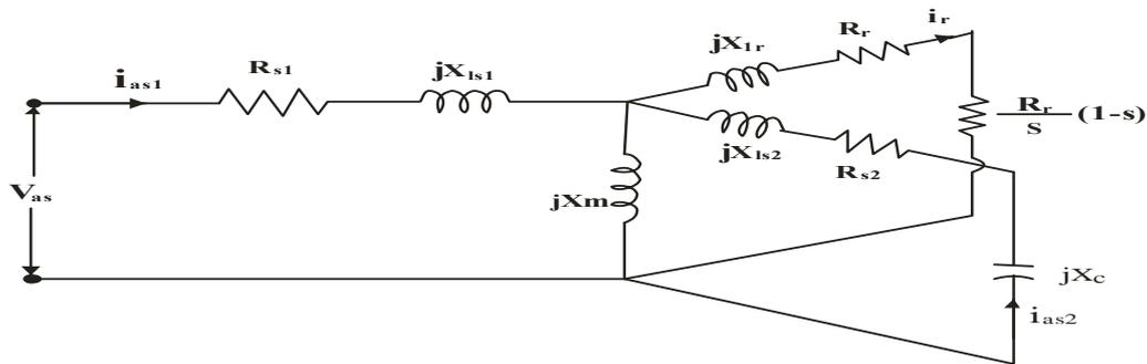
Figure 2. Steady State Equivalent Circuit.
