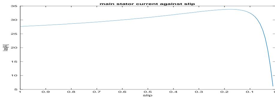
Fig 4. Main Stator Current Against Slip
