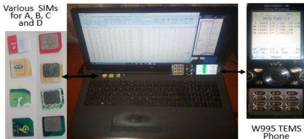
Figure 1: The experimental set-up of W995 Ericson with built-in TEMS software.
