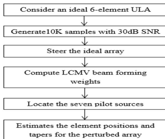
Figure 1: Steps of pilot calibration method for antenna array.
