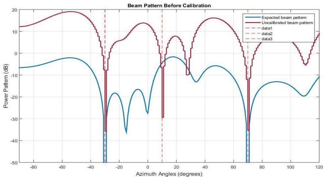
Figure 3: Beam pattern for an array of  $N = 6$  element before array calibration under  $SNR = 30$  dB.
