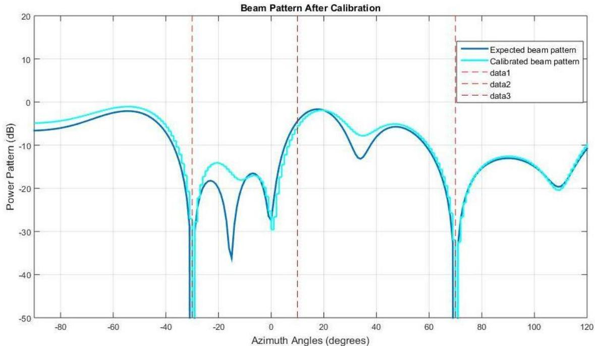
**Figure 4:** Beam pattern for an array of  $N = 6$  element after array calibration under  $SNR = 30dB$ .
