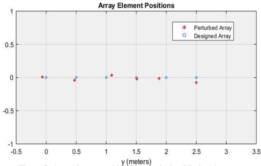
Figure 2: Array element position for perturbed and designed array.
