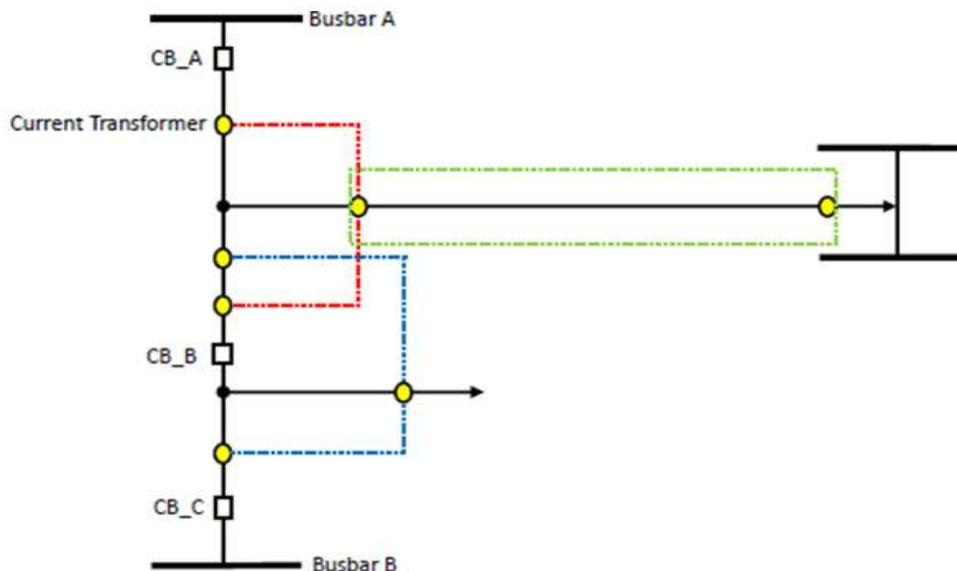
**Figure 2.1: Field Differential Protection & Line Differential Protection Scheme**
