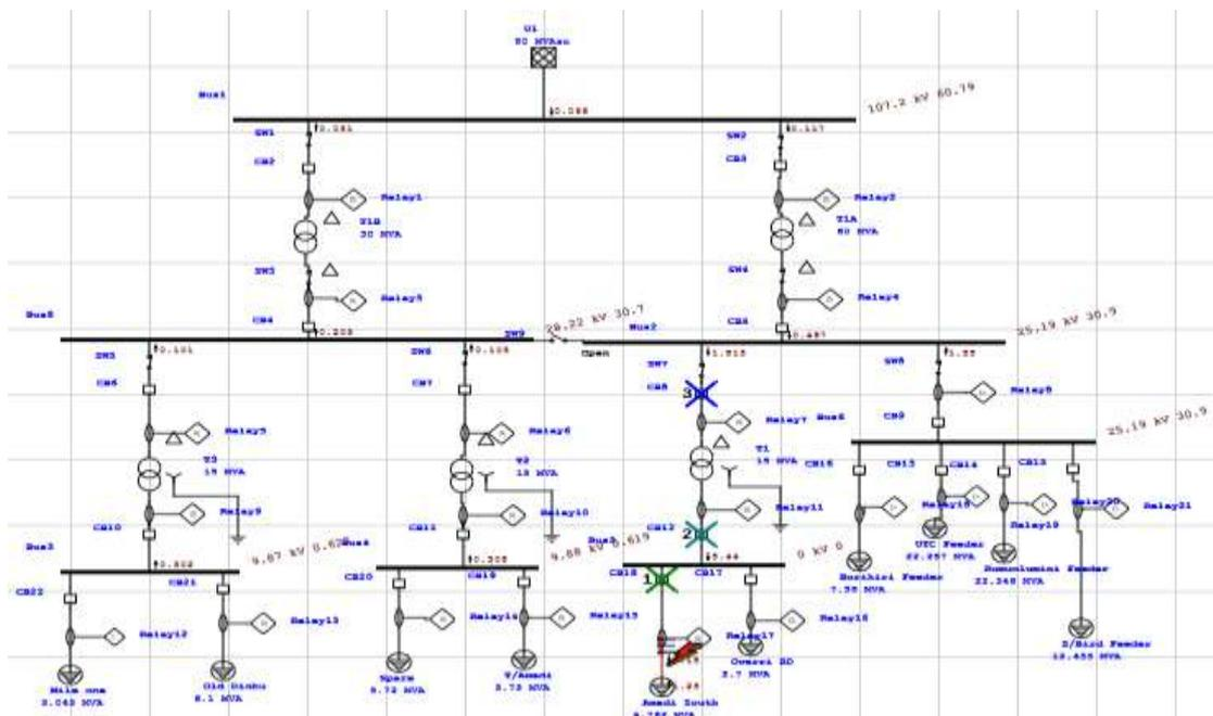
**Figure 4.1: Presentation of Simulated Single Line Diagram Showing Fault on Amadi South 11KV Feeder**
