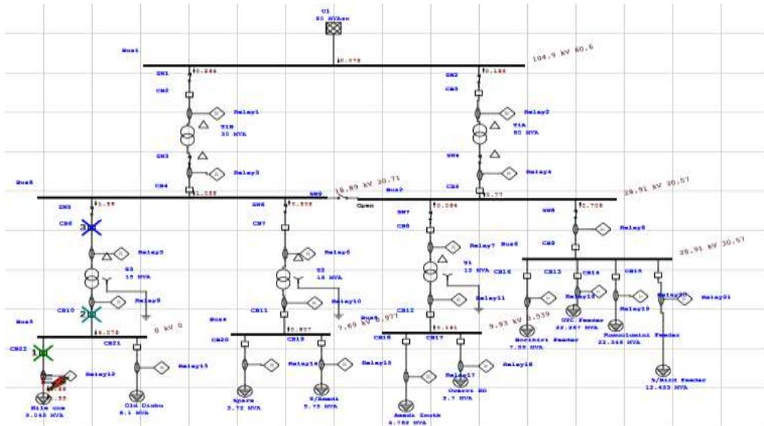
Figure 4.2: Presentation of Simulated Single Line Diagram Showing Fault on Mile One 11KV Feeder
