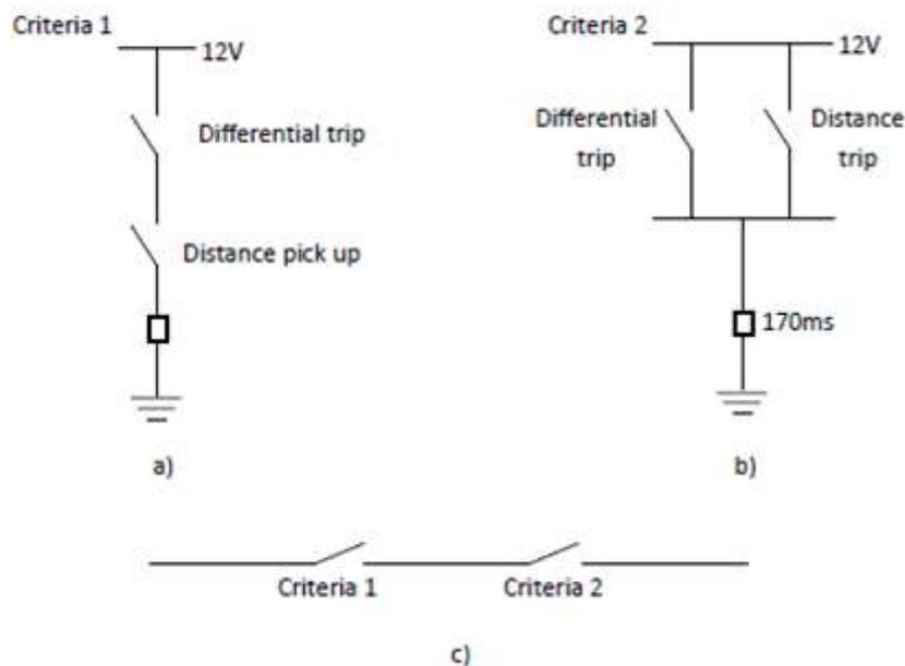
Figure 2.3: Circuit Breaker Failure Function Criteria
