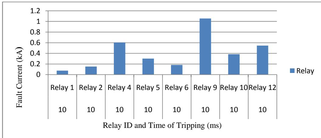
**Figure 4.5: A Bar Chart of Symmetrical 3-Phase Faults of Relay ID and Time of Tripping at 10 (ms) with Faults Current**
