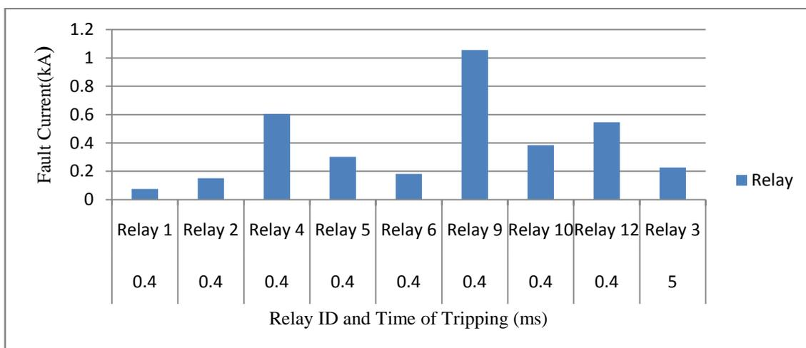
Figure 4.4: A Bar Chart of Symmetrical 3-Phase Faults of Relay ID and Time of Tripping at 0.4 (ms) with Faults Current
