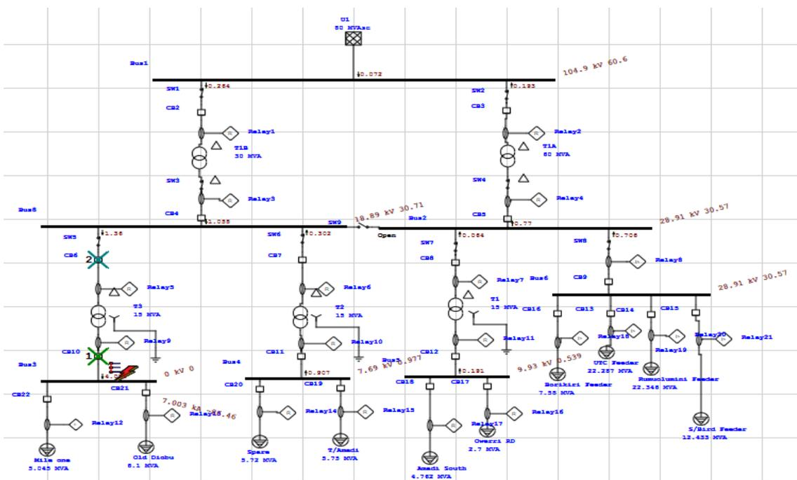
Figure 4.3: Presentation of Simulated Single Line Diagram Showing Fault on Transformer T1 11KV Incomer
