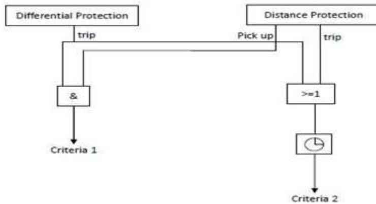
Figure 2.2: Circuit Breaker Failure Function Principle
