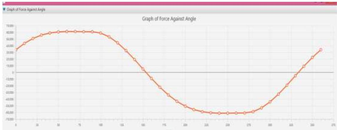
Figure 4:Plot of Total Wave Force against Wave Phase Angle
