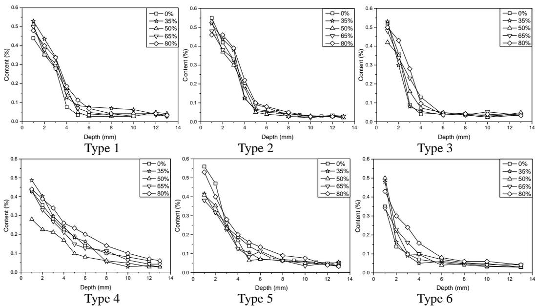
**Fig. 4:** Chloride profiles as determined in concrete exposed to 5 % NaCl solution for 60 days
