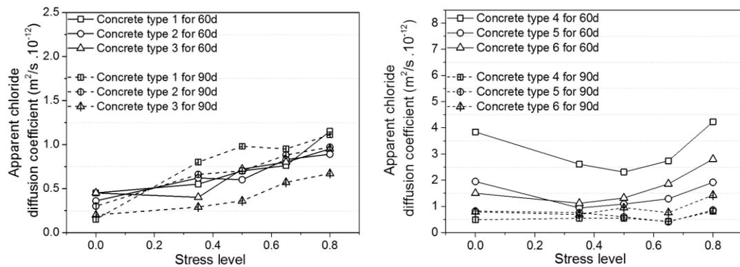
Fig. 6: Apparent chloride diffusion coefficient  $D(x)$  at different stress levels for slag concrete activated by NaOH (left) and water-glass (right).
