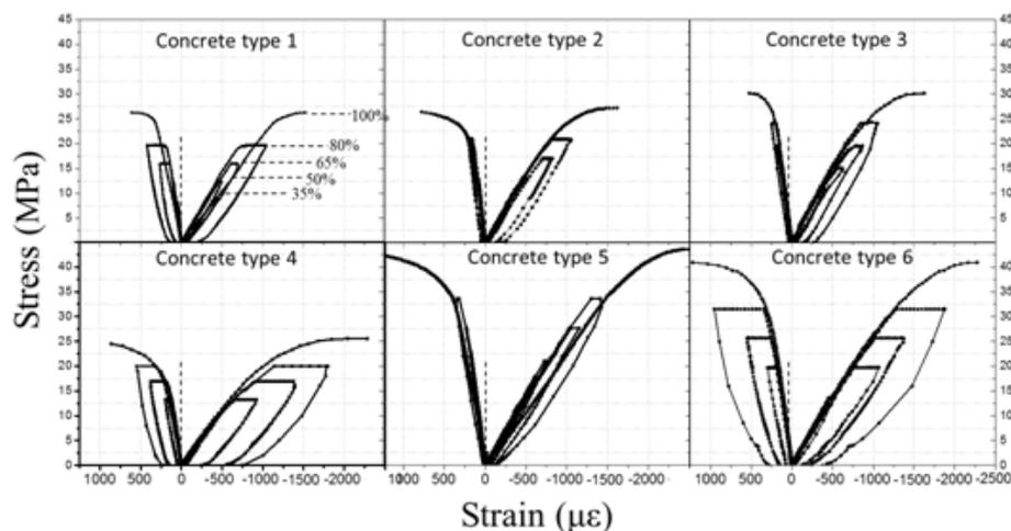
Fig. 2: Stress-strain diagrams as obtained on prisms of all six types of concrete. The negative strain corresponds to deformation in the direction parallel to the applied load (shortening), while the positive strain corresponds to the lateral deformation (extension). Five different stress levels, namely 35%, 50%, 65%, 80%, and 100%, were applied on all concrete prisms, as indicated in this figure for concrete type 1.
