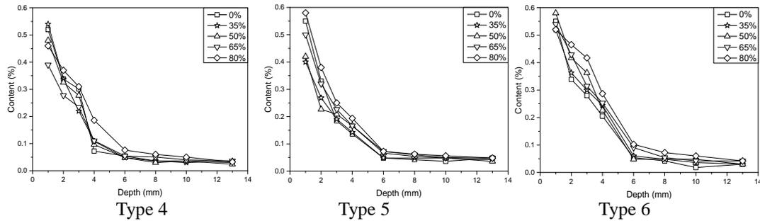
Fig. 5: Chloride profiles as determined in concrete exposed to 5 % NaCl solution for 90 days
