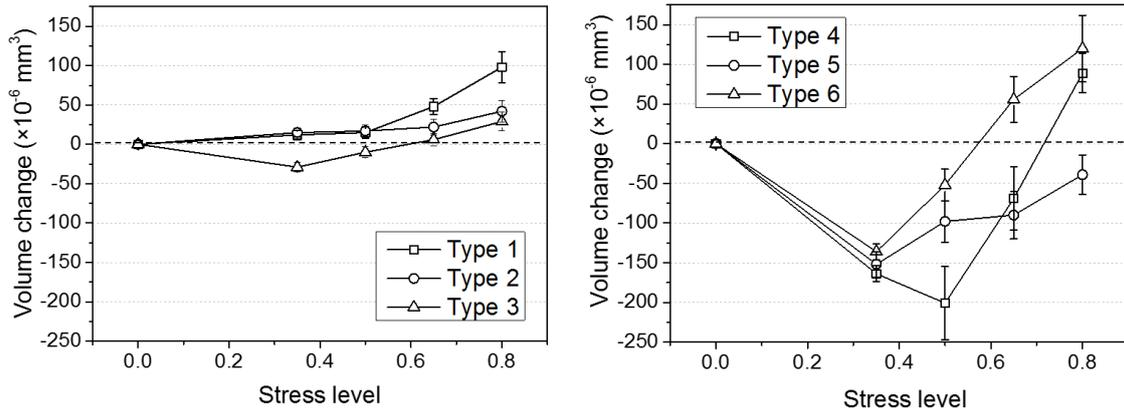
**Fig. 3:** Volumetric change as observed after unloading of preloaded cubes as function of the applied stress level for concrete activated with NaOH (left) and with water-glass (right).
