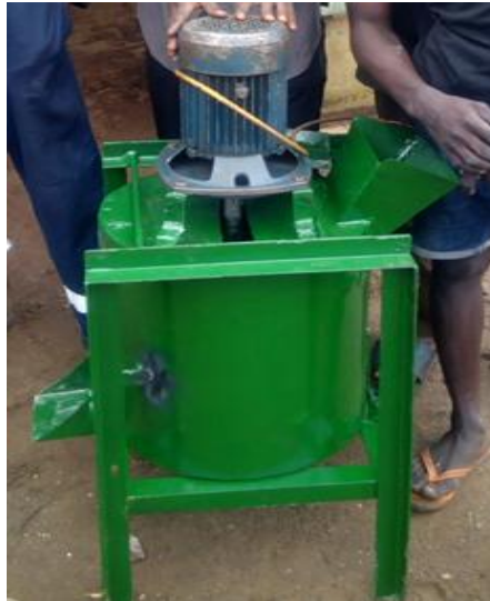
Plate 2. Fabricated motorized oil palm fruit rotary digester machine
