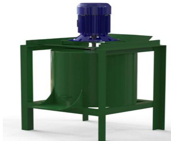
Fig. 3 Isometric modeled view of the motorized oil palm fruit rotary digester machine
