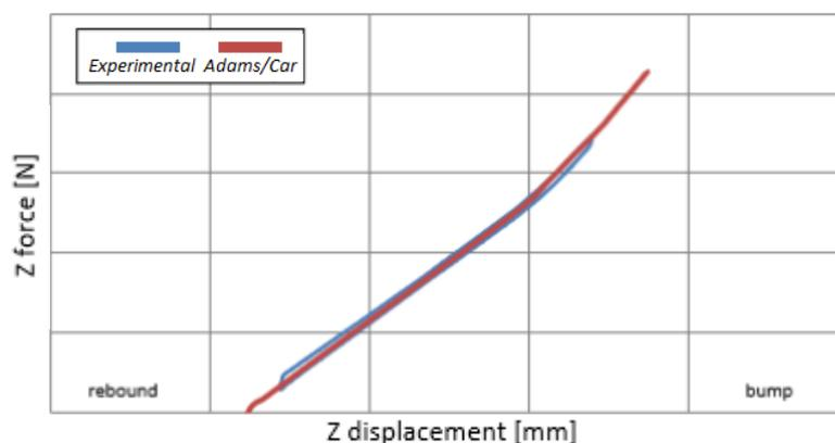
Fig.5. RF Wheel rate in opposed test
