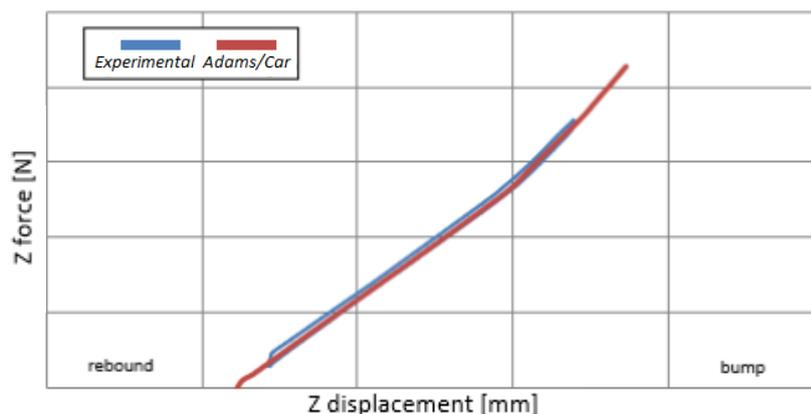
Fig.4. LF Wheel rate in opposed test
