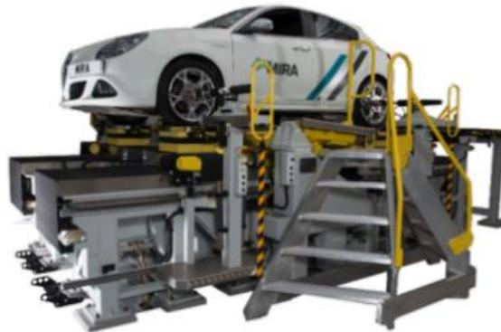
**Fig.3. Suspension parameter measurement machine**
