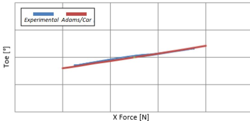
Fig.9. LF toe compliance in lateral test
