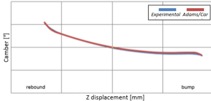
**Fig.6. Bump camber in parallel test**
