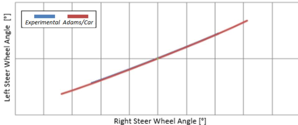
Fig.11. Ackermann in steering test
