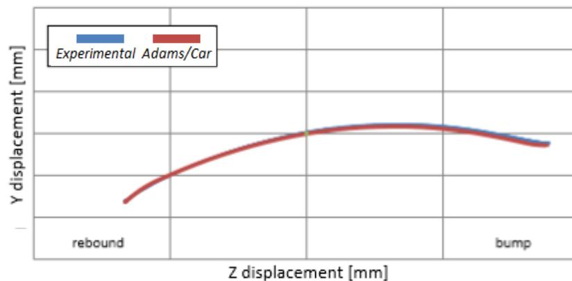
**Fig.7. Bump camber in parallel test**
