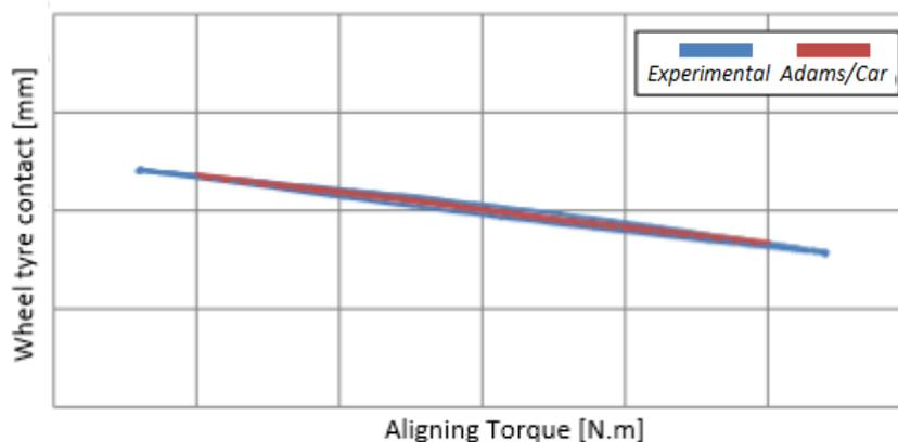
Fig.10. LF ground-tire compliance in aligning test
