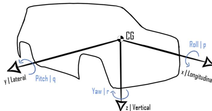
Fig.2. SAE coordinate system
