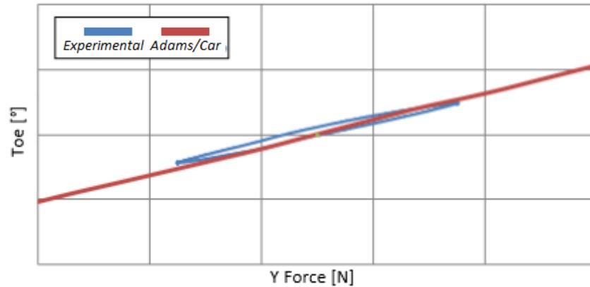
Fig.8. LF toe compliance in lateral test
