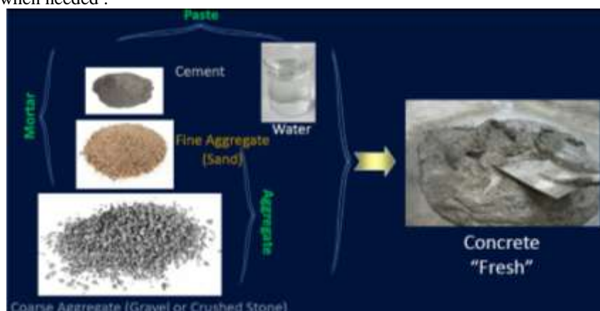
Fig.1. Main constituents of concrete.
