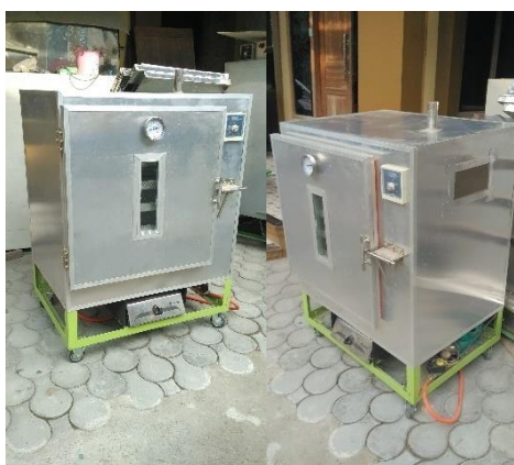
Fig. 2. "Cabinet"-type Clove (or other agriculture produce) Dryer.
