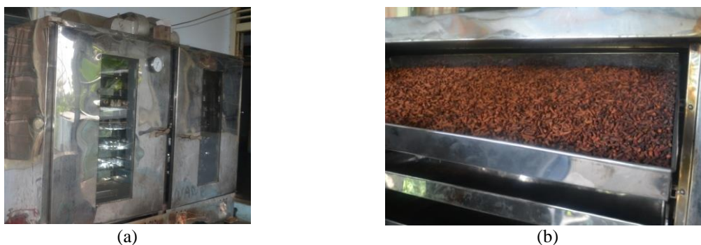
Fig. 1. (a) Clove bud dryer, arranged as several levels of pan, (b) one of pan filled with clove buds.
