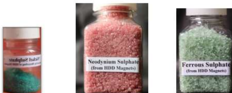
Fig. 6(a) Nickel Sulphate, (6b) Neodymium Sulphate and (6c) Ferrous sulphate
