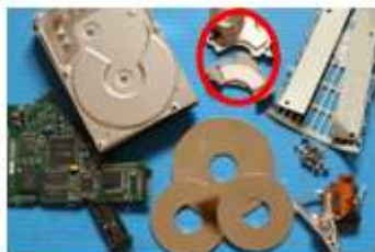
Fig.2 Exploded view of HDD
