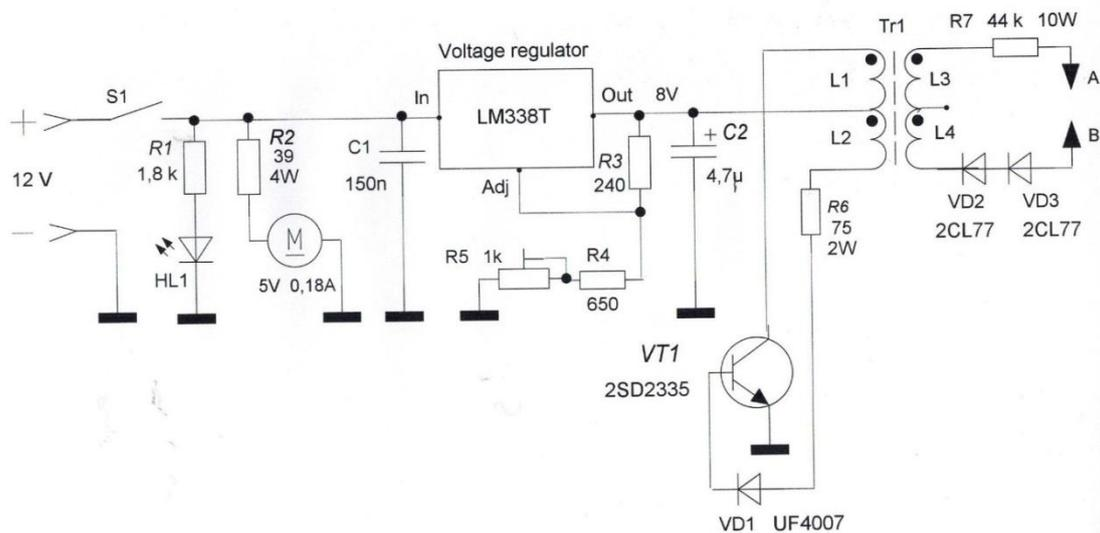
**Fig.3.** Electrical circuit of the device for the demonstration of the Lorentz force using a spark discharge.
