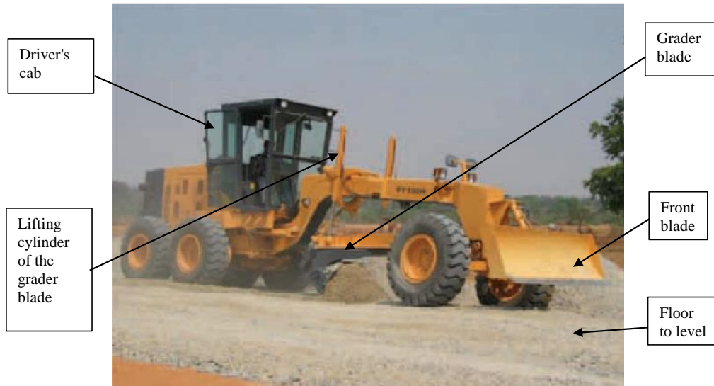
Fig. 2. Grader operating in a building site
