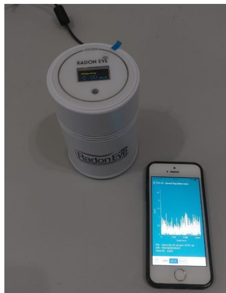
Fig.02. Data collection of RadonEye RD200 with an Iphone
