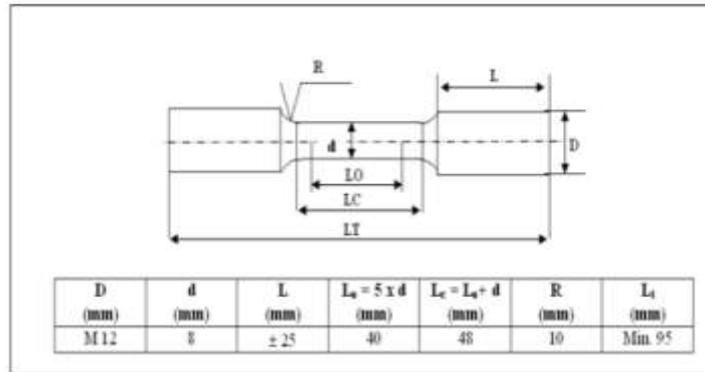
Fig. 2: Dimensions of the test specimen [11].
