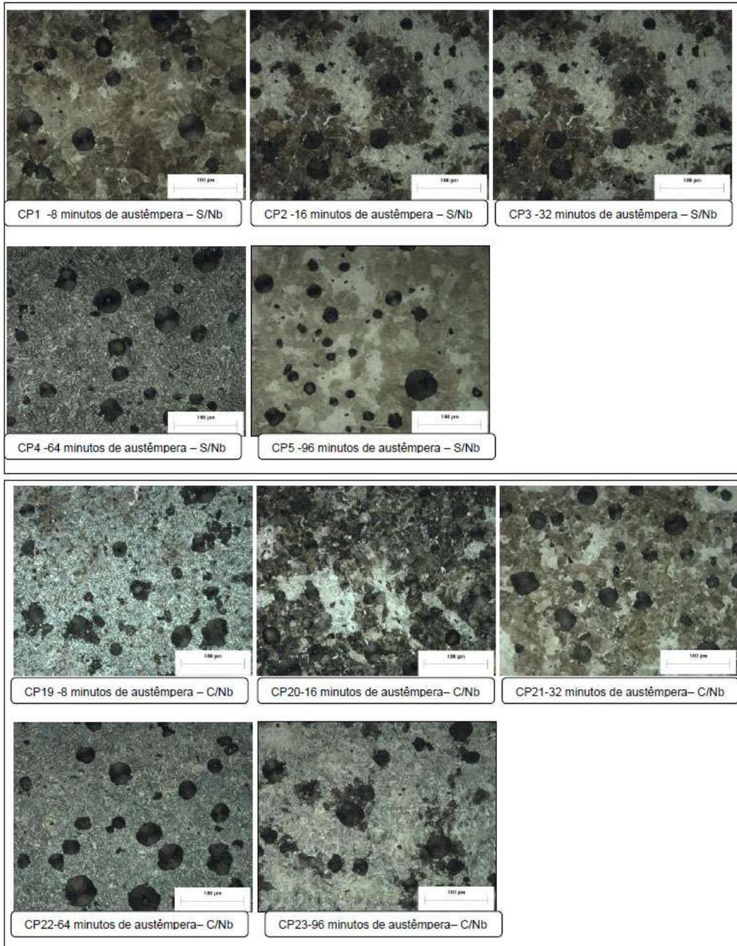
**Fig. 7: Metallographic analysis of the samples without and with addition of niobium and with chemical attack, 500x of magnification.**
