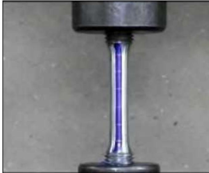
Fig. 4: Fixation of the specimens for the tensile test.
