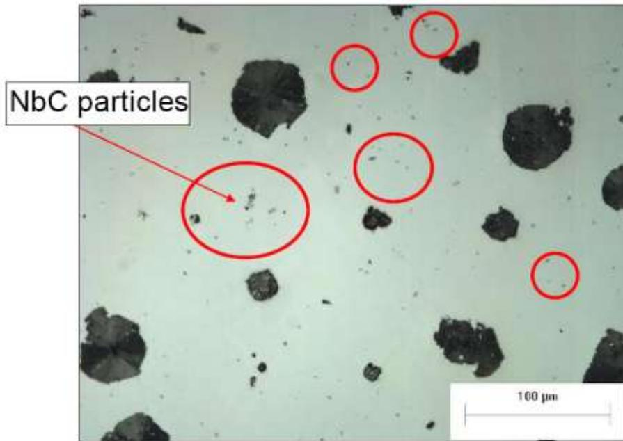
Fig. 8: NbC particles dispersed in the sample matrix.
