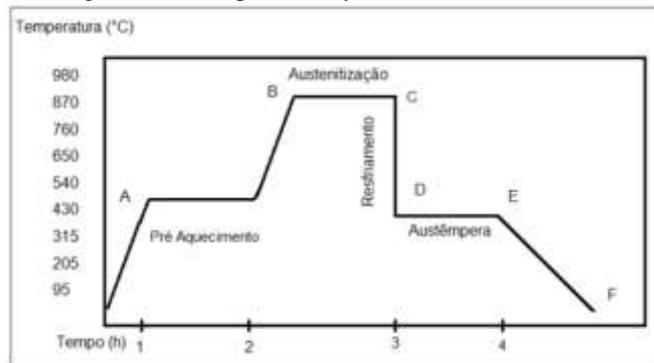
Fig. 3: Austempering thermal treatment.
