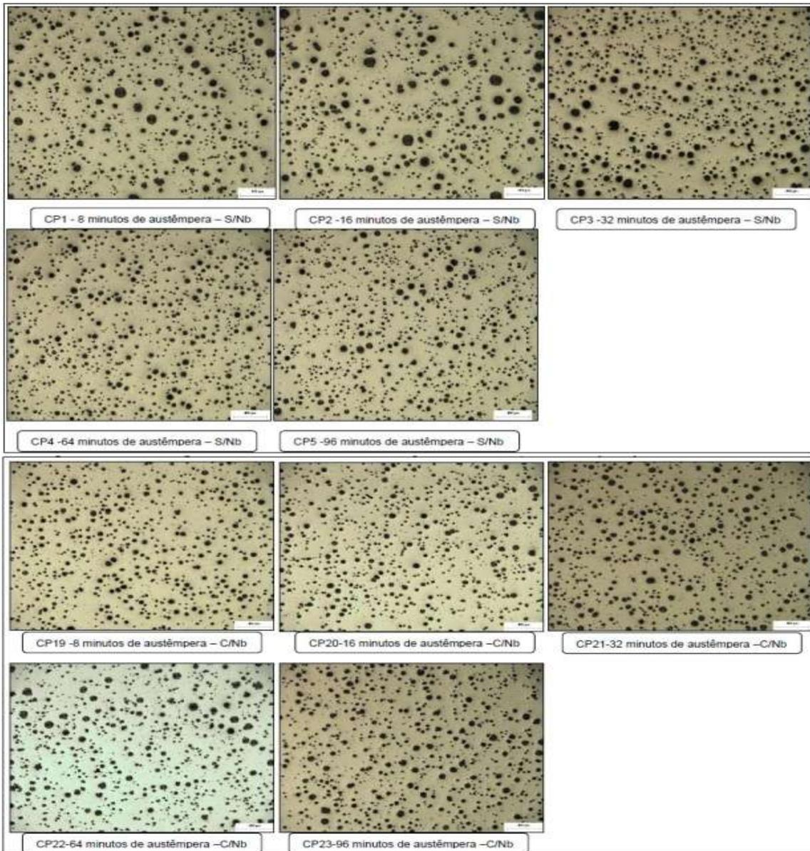
**Fig. 5: Metallographic analysis of samples without addition of Nb and without chemical attack, 100x of magnification.**
