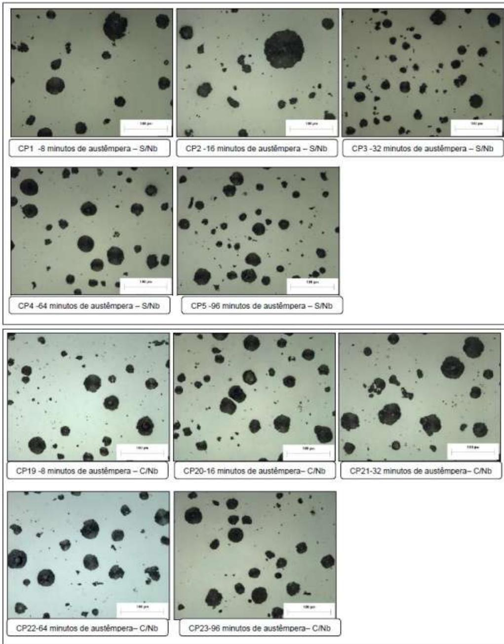
**Fig. 6: Metallographic analysis of samples without addition of Nb and without chemical attack, 100x of magnification.**
