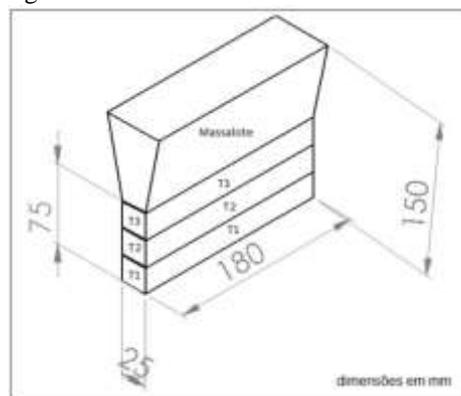
Fig. 1: Dimensions of Y-type block [11].
