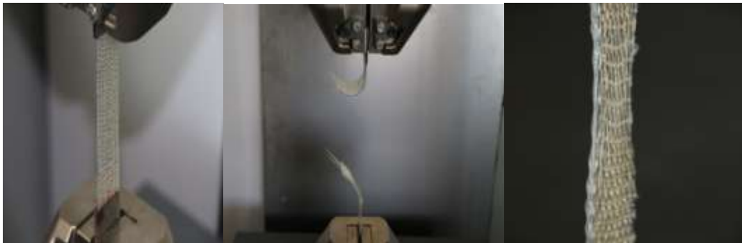
Figure 4. Tensile testing process for composite material samples
