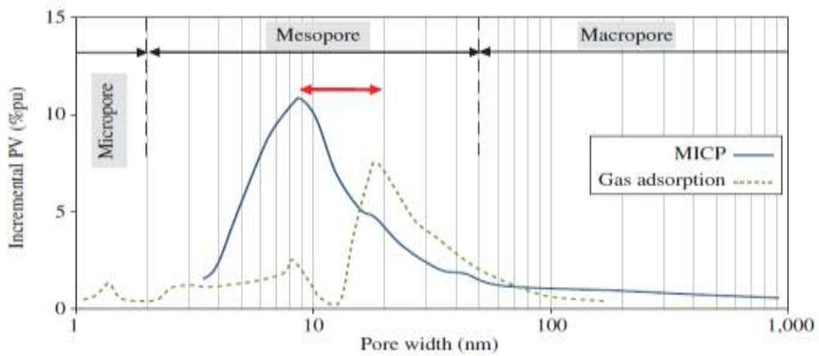
Figure 5: A comparison between MICP and gas adsorption data for shale gas sample (Q. Wang et al., 2018)
