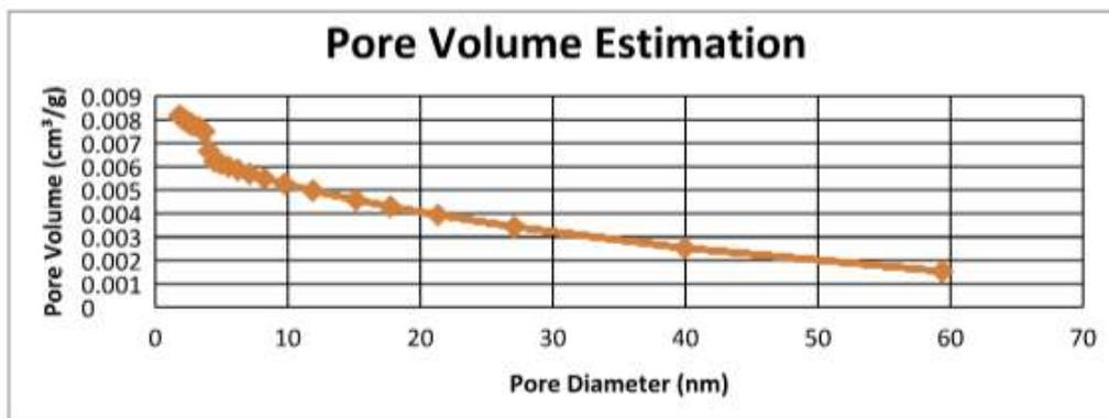
Figure 16: Pore Volume Estimation of Batu Gajah Samples
