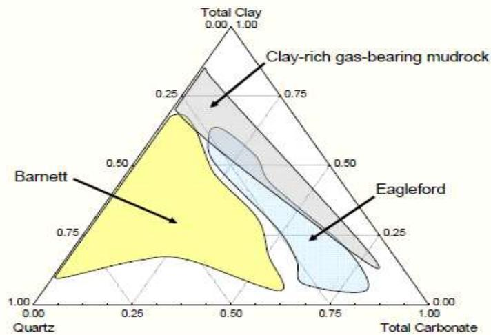
Figure 2: Mineral compositional of shale gas reservoirs (Alyousuf et al., 2011)
