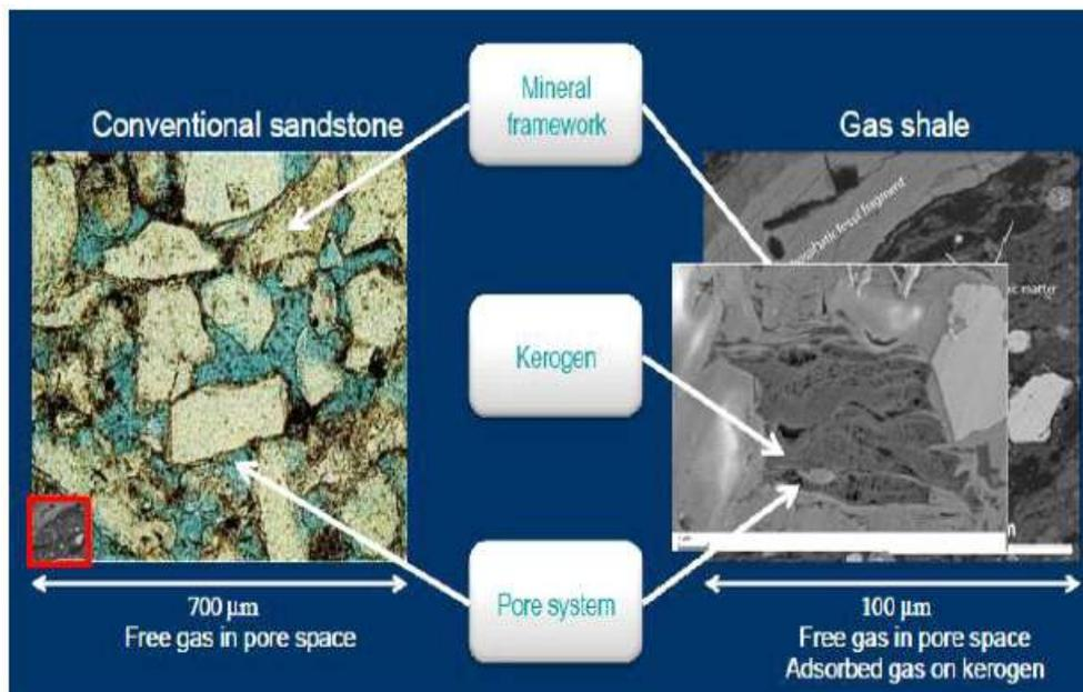
Figure 6: Pore space in sandstone and shale (P. Wang et al., 2018)
