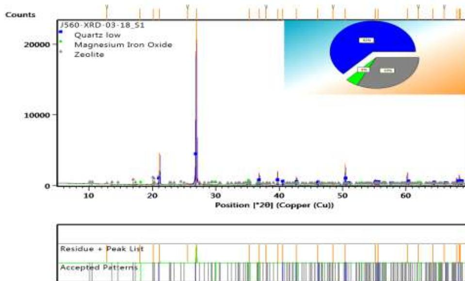
Figure 7: Mineralogical component of Kedah samples
