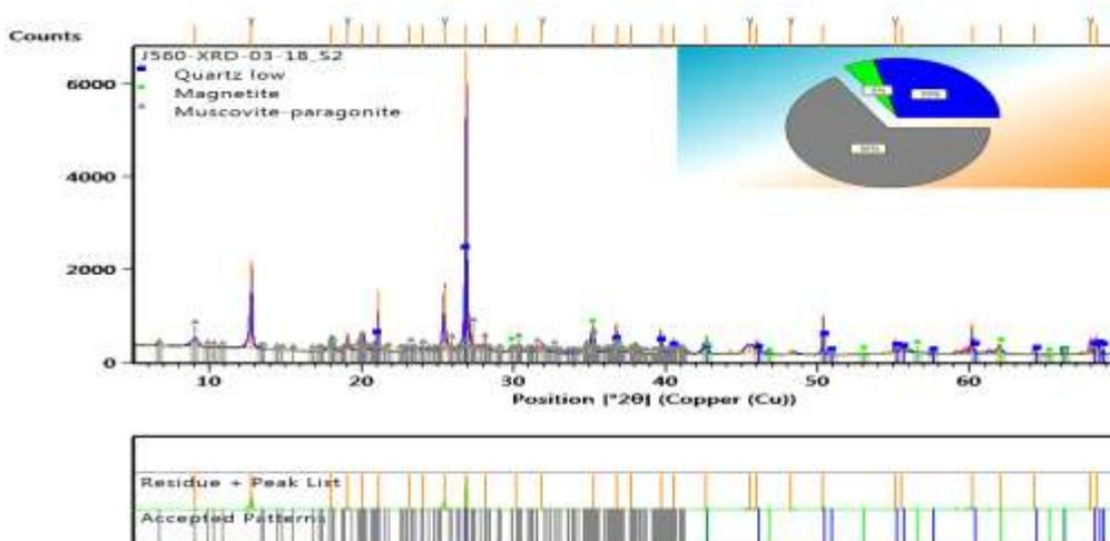
Figure 9: Mineralogical component of Batu Gajah samples
