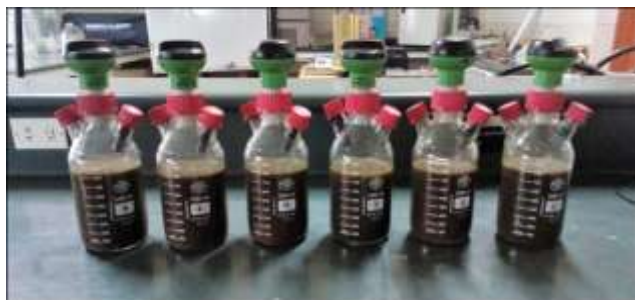
Figure 2. OxiTop® Control measuring equipment
