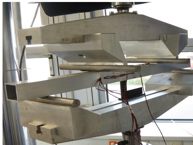
Fig. 6: Test rig for the four point bending test
