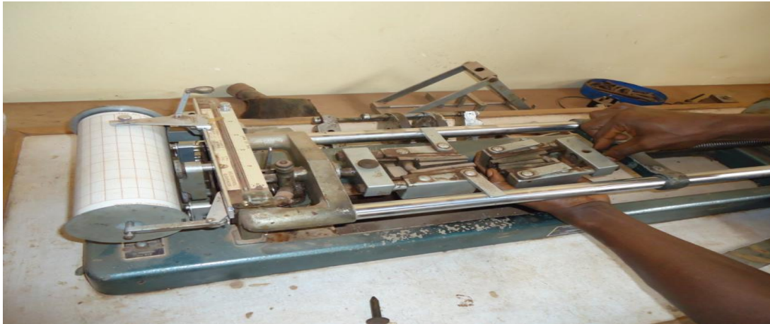
Fig. 2: Hounsfield Monsanto Universal Tensometer
