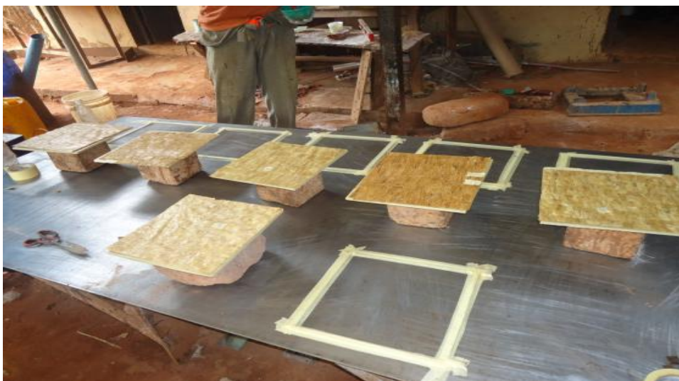
Fig. 1: Mould set-up for fiber-reinforced composites, CCRD, Nsukka
