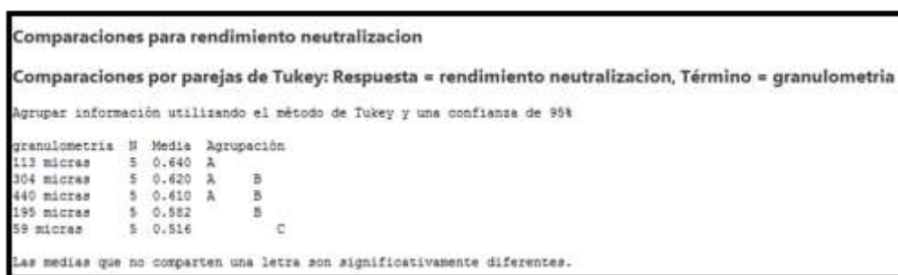
Figure 2. It is observed in the figure that natural dolomite with a granulometry of 113, 304 and 440 microns are classified in group A with the highest neutralization yields of 64%, 62% and 61% respectively, and they are statistically similar.
