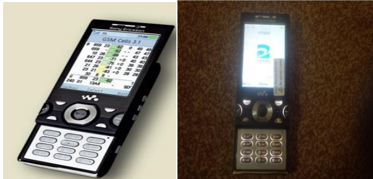
Figure 1.0: W995 Sony Ericsson Test Phone with built-in TEMS (TEMS POCKET)
