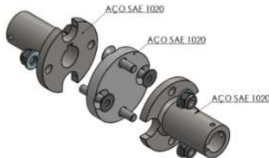
Figure 12- Exploded view of the rigid coupling with SAE 1020 steel disk
