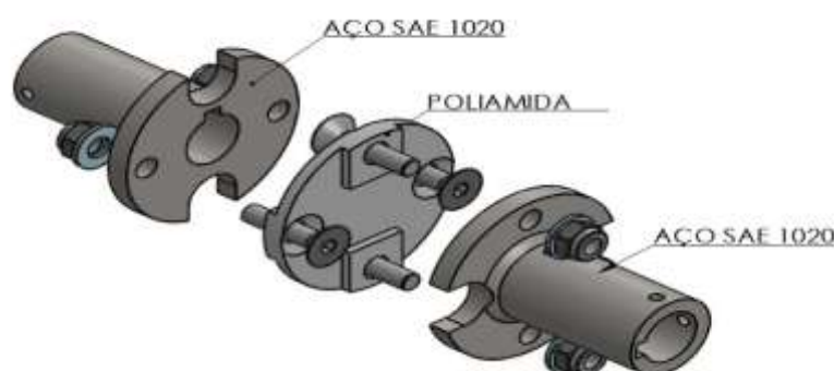
Figure 11 – exploded view flexible coupling with polyamide
