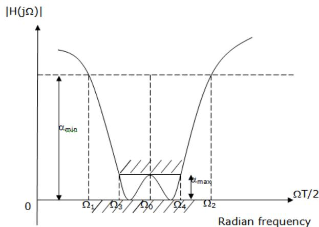
**Figure 3:** Magnitude Response of Bandstop Filter with Normalized Frequency  $\Omega$  or  $\Omega T/2$
