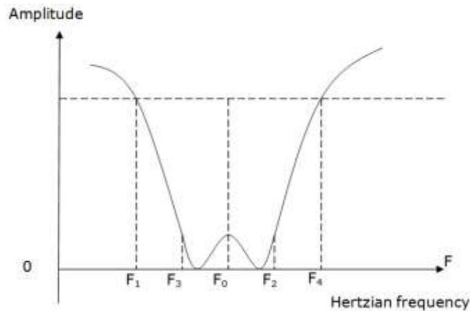
**Figure 2:** Amplitude Response of Bandstop Filter
