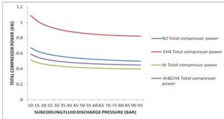
**Fig. 9.**Sub-cooling fluid discharge pressure versus compressor duty requirement curves.
