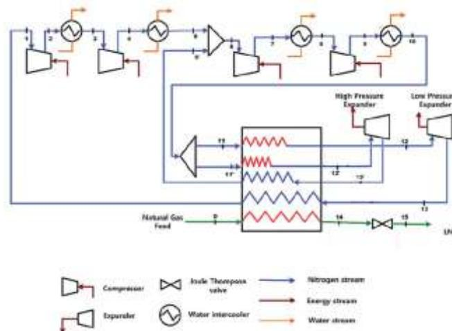
Fig. 2. A schematic of a dual expander natural gas liquefaction process (Adapted from Khan et al, 2015).
