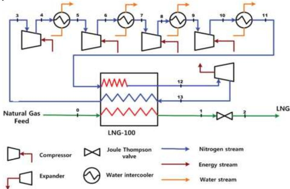
Fig.1. A schematic of a single expander natural gas liquefaction process (Adapted from Khan et al, 2015)
