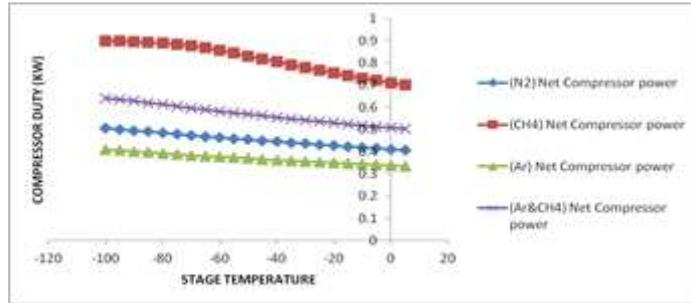
Fig. 3. Compressor duty values as a function of stage temperature for the four refrigerant options.
