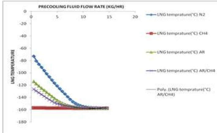
Fig.6. Precooling fluid flow rate versus produced LNG temperature
