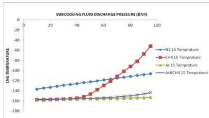
**Fig. 10.**Sub-cooling fluid discharge pressure versus LNG temperature profiles.
