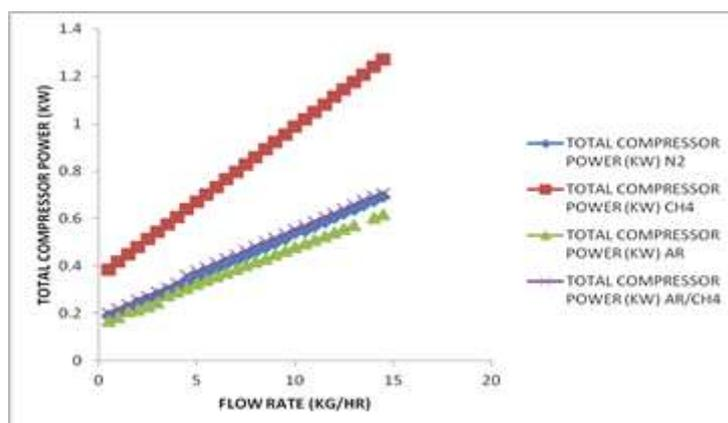
Fig. 5. Precooling fluid flow rate versus total compressor power requirements.
