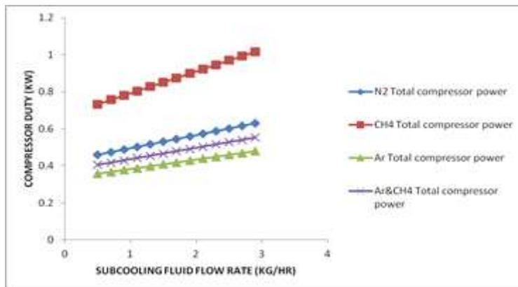
Fig. 7. Sub-cooling fluid flow rate and compressor duty profiles
