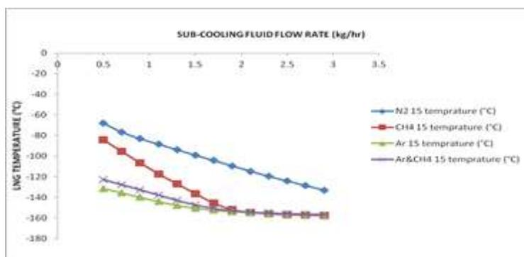
Fig. 8. Sub-cooling fluid flow rate versus produced LNG temperature profiles
