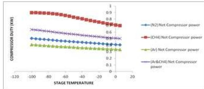
Fig. 3. Compressor duty values as a function of stage temperature for the four refrigerant options.
