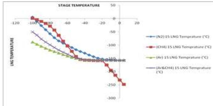
Fig. 4. LNG temperature values as a function of stage temperature for the four refrigerant options.
