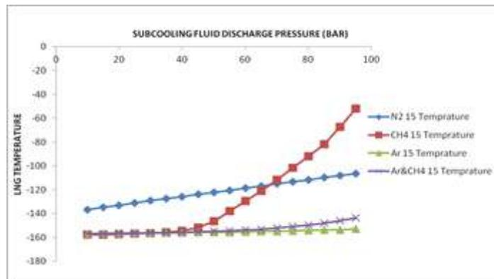
**Fig. 10.**Sub-cooling fluid discharge pressure versus LNG temperature profiles.
