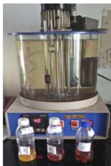
Figure 4. Kinematic viscosity test at 40^{\circ}\text{C}
