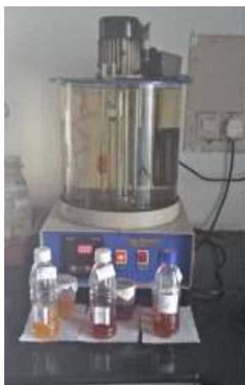
Figure 4. Kinematic viscosity test at 40^{\circ}\text{C}
