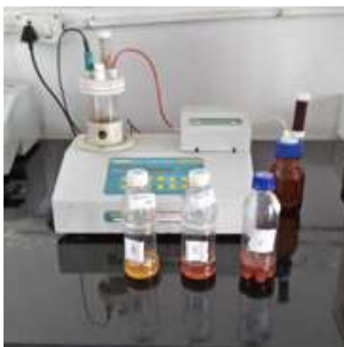
Figure5. Experimental setup for water content test
