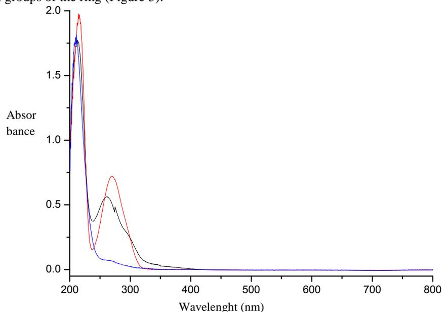
Fig. 5 UV-visible spectrum of 1 (black), gallic acid (red) and bromobutane (blue)
