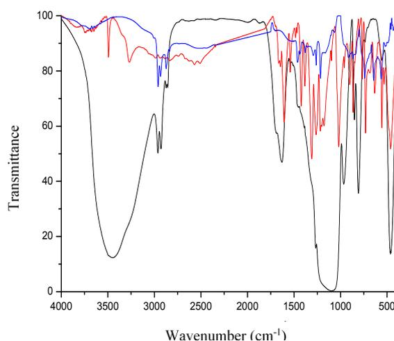
Fig. 3 FTIR spectra of 1 (black), gallic acid (red), bromobutane (blue)
