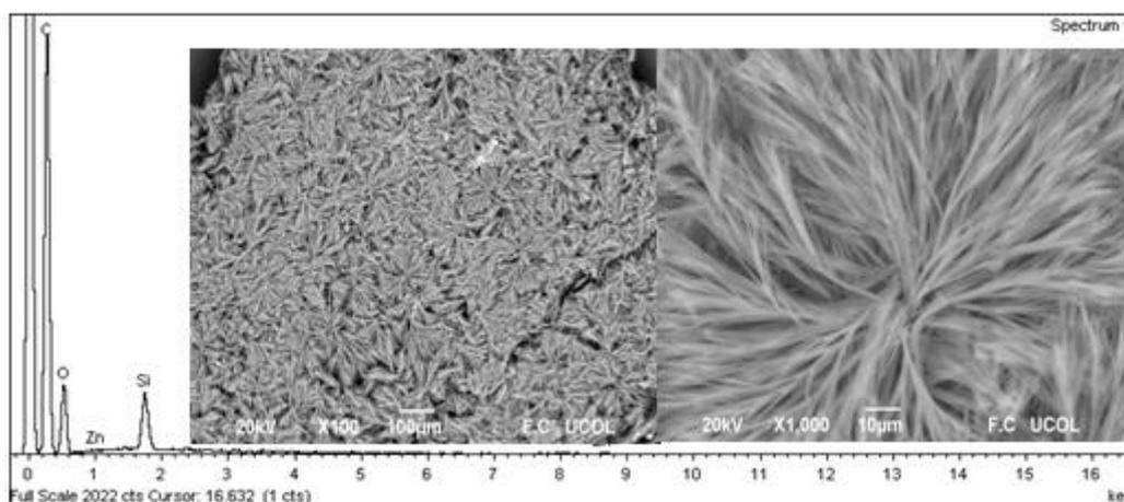
Fig. 7 Morphology of 3,4,5-tributoxy ethyl benzoic acid (2) by SEM-DS
