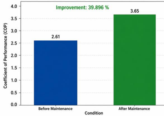
Figure 2: COP Improvement After Preventive Maintenance
