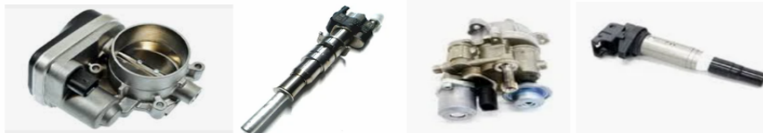
Fig.4 Images of Actuators in SI Engine - Electronic Throttle Control, Fuel Injectors, Fuel Pump and Ignition Coil (Actuators)
