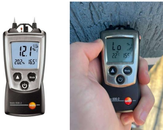
Fig. 2. TESTO 606-2 material temperature and moisture measuring instrument
