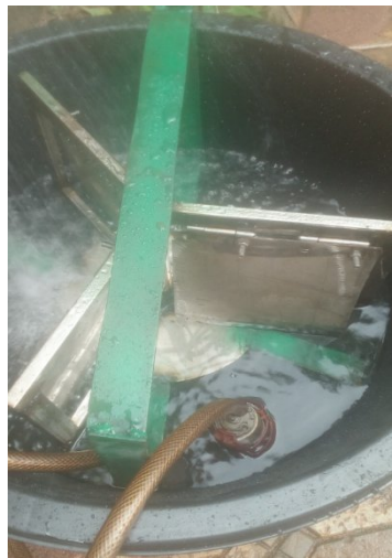
Figure 2 Experimental Vertical Tidal Current Turbine.
