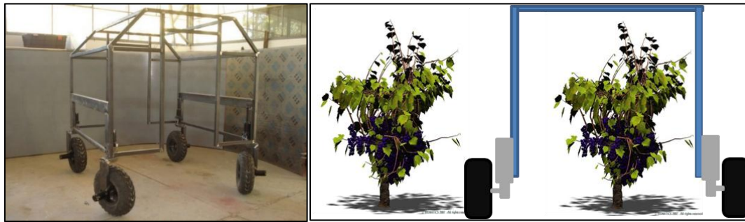
Fig. 1. Structure of the robot BACO and its position on the row.
