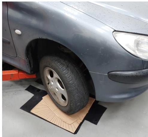
Figure 3 – Manual experimental procedure for measuring the steering angle during class.
