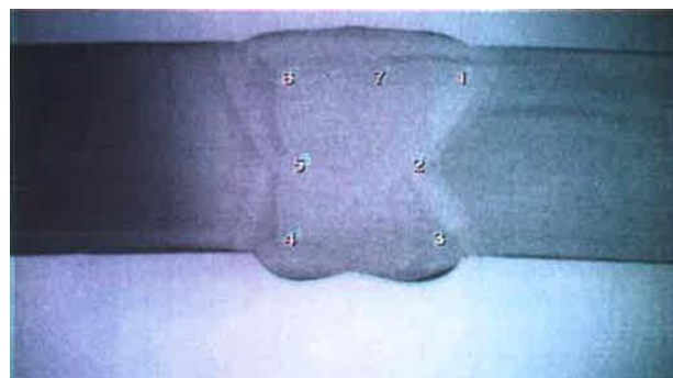
Figure 5: Vickers test according to ASTM E 384.
