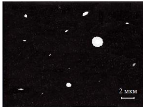
Fig. 3. General view of impurity accumulations of nickel in silicon.
