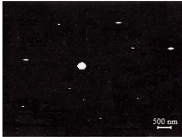
Fig. 1. General view of cobalt impurity nanoclusters in silicon.
