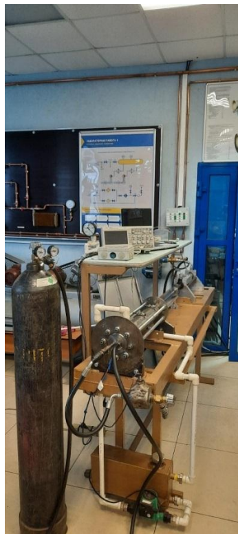
Figure 4— An experimental stand with a slow-moving long-stroke stage
