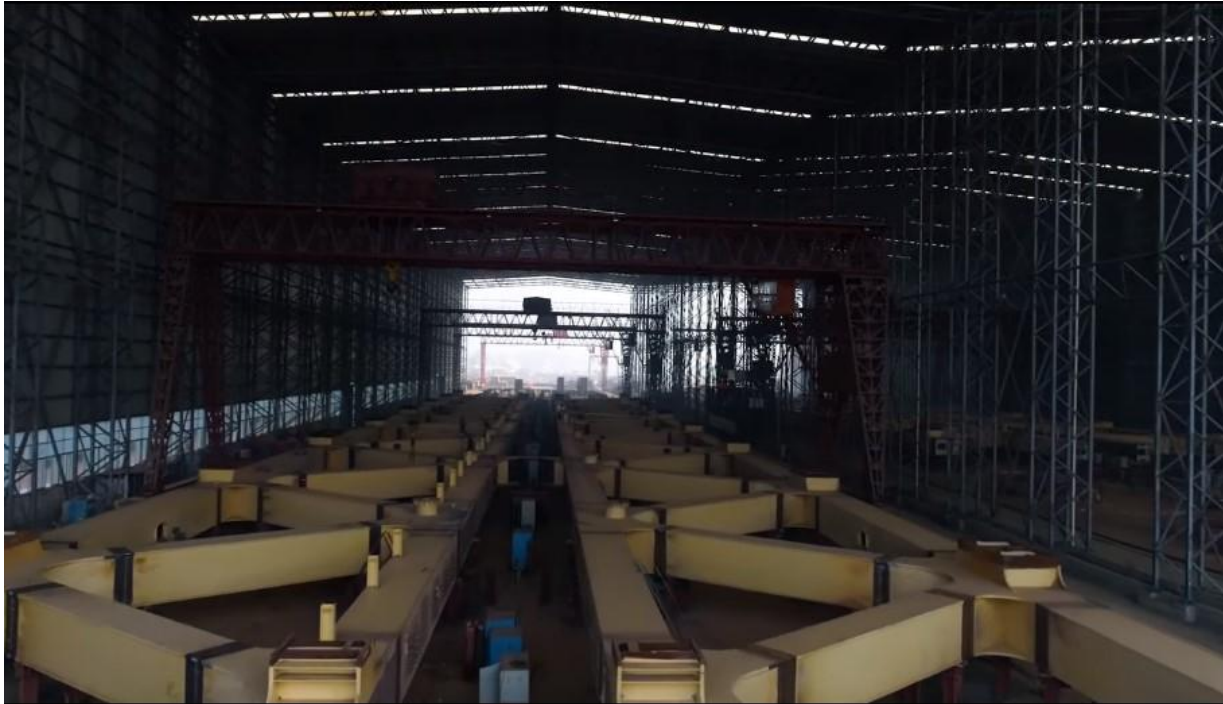
Figure 9: Typical Parts of Main Bridge Warren Trusses
