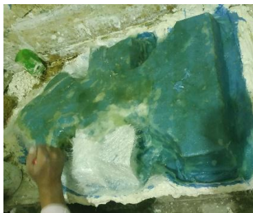
Image ( 19 ) shows Re-pour a layer of polyester onto the reinforcement fibers
