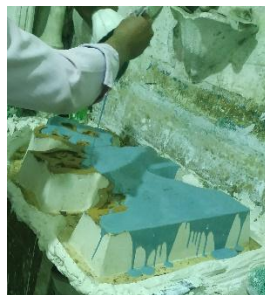
Image (14) shows the polyester casting on the surface of the model
