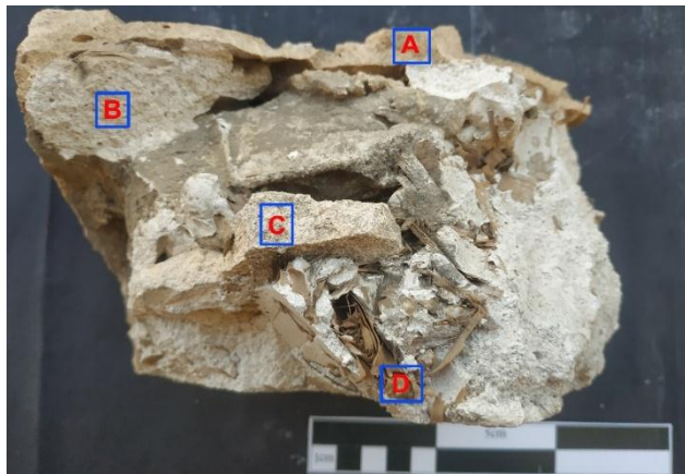
Image (6) A outer surface , B inner mortar , C filler stone aggregate , D reinforcement plant material .
