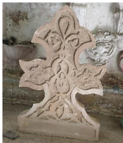
Image (10 ) shows an sharrafa of the artificial stone for which a mold will be made
