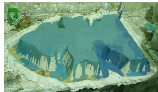
Image (15 ) shows the polyester casting on the surface of the model
