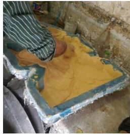
Image ( 26) shows Distribution of cast material
