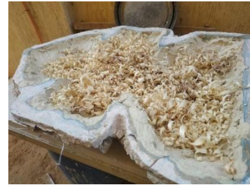
Image ( 27 ) shows Adding sawdust to the components of the sharrafat
