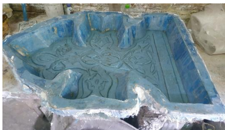
Image (22 ) shows Completion the polyester mold
