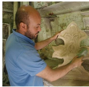
Image ( 11) shows an sharrafa Cleaning before making the mold
