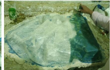
Image (18 ) shows Re-pour a layer of polyester onto the reinforcement fibers
