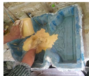
Image (24 ) shows The process of pouring the first surface layer that gives the shape of the decoration
