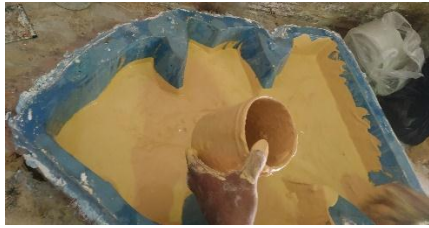
Image ( 25) shows Distribution of cast material
