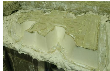
Image ( 12) shows Adjust the sides to make it easier to remove the mold
