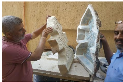
Image ( 29) shows Detachment of the casted sharrafa from the mold
