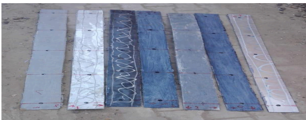
Figure 3: laminates that used to strengthen of beams
