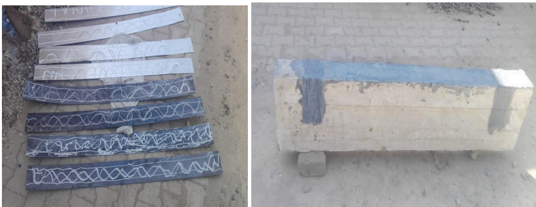
Figure 2: laminates that used to strengthen of (SB4 CFRP) and (SB9 GFRP) beams
