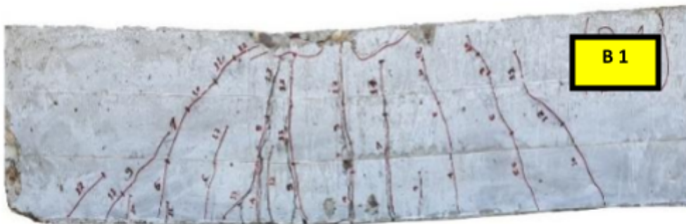
Figure 6: Failure mode and pattern of cracks for SBC-control beam
