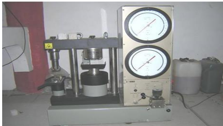
Fig 4. Mortar Compressive Strength Test Equipment
