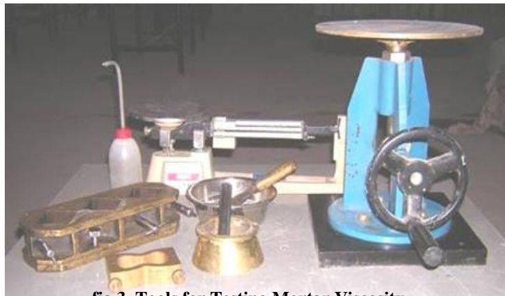
fig 3. Tools for Testing Mortar Viscosity
