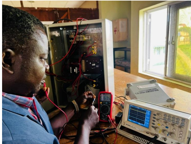
Fig. 3. Experimental testing of the developed auxiliary DC supply system
