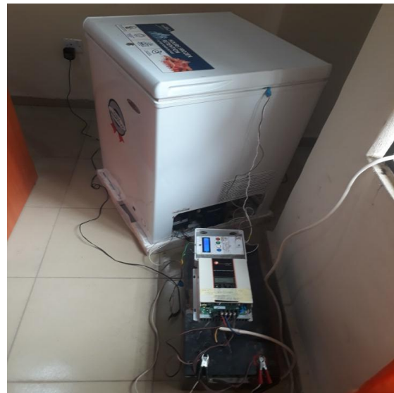
Figure 11: The Complete Design using 100Ltr Thermocool Deep Freezer
