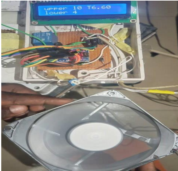
Figure 8: Fridge Temperature is 6°C Compressor Running
