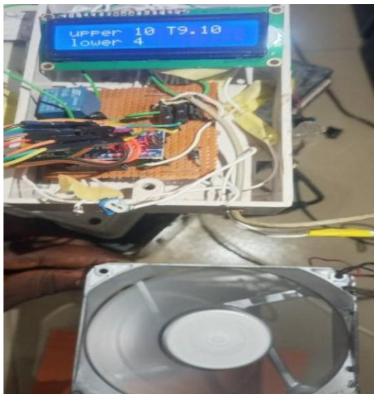
Figure 10: Compressor Turns On as Temperature Rises to Upper
