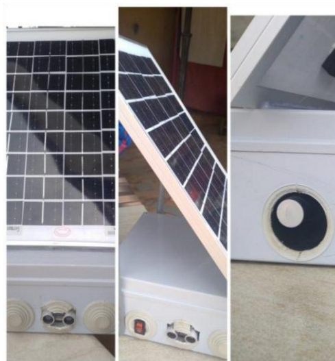
Figure 2: Ultrasonic Bird repellent case and solar panel
